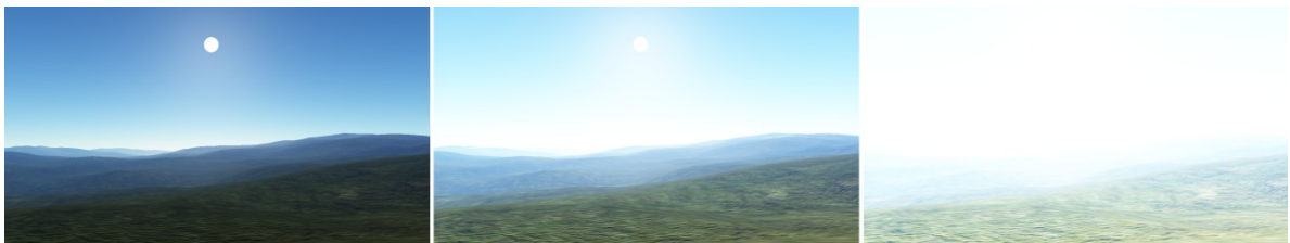
Figure 4-42: Tone mapping with different settings for exposure value: (left) exposure = 1 (middle) exposure = 3 (right) exposure = 10.
